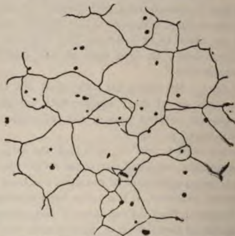
FIG. 8.—TRANSVERSE SECTION OF SWEDISH BAR IRON. Carbon 0%. Magnified 230 diameters.
